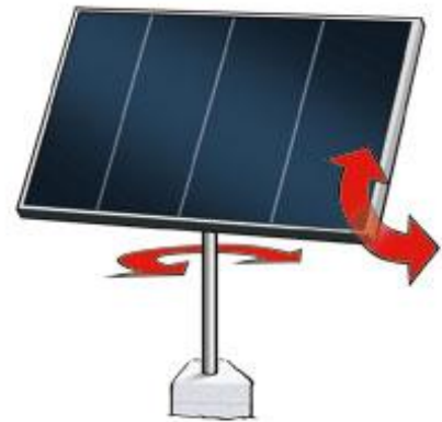
Figure A1 2: A solar-PV panel with two degrees of freedom in its' movements.
